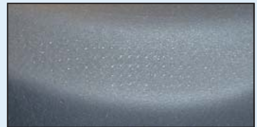
Inverted Head Radius of a Top-Hat Diaphragm.
